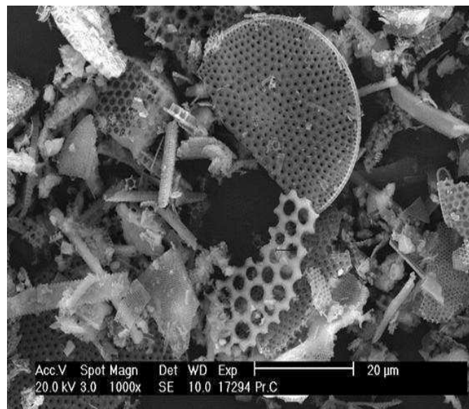
Fig. 3 SEM micrography of the diatomite powder
