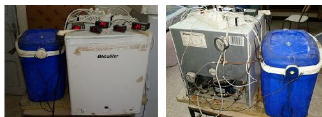
Fig.2: Domestic Refrigerator with Water Heater Tank photograph.
